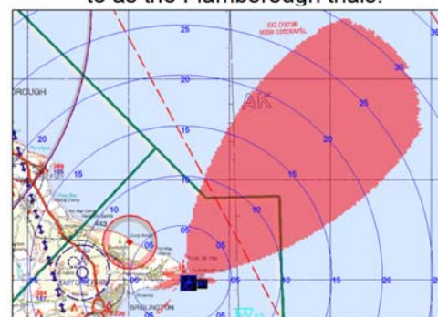
Figure 4: Jamming Zone During Trials Conducted by the General Lighthouse Authorities (GLA) of the U.K. and Ireland (Last, 2010). These are referred to as the Flamborough trials.
