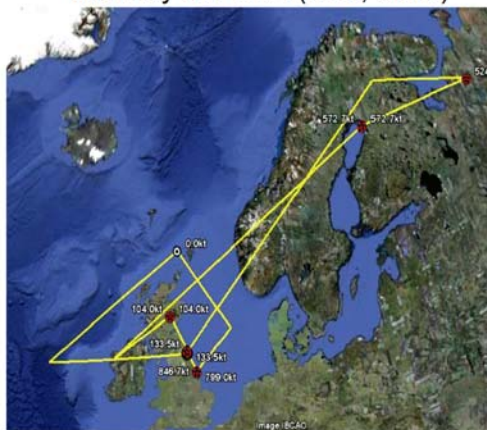
Figure 6: Position Fixes Induced by a Low Power Jammer Placed on Board the THV Galatea During Trials by the GLA (Last, 2010)
